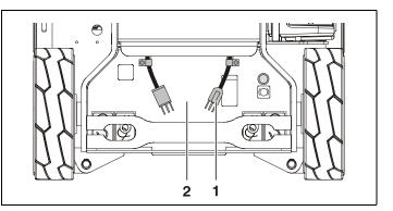
Figure 4-1. Location of Battery Charger AC Input Plug
