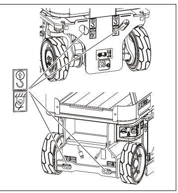
Figure 4-13. Tie Down and Lift Lug Locations.
