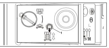
Figure 4-7. Lowering Platform From Ground Control
