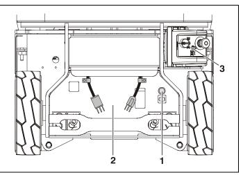
Figure 3-6. Location of Brake Release Switch (Rear of Machine)
