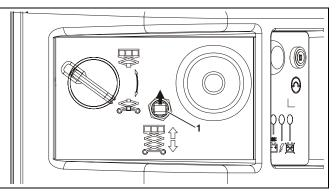
Figure 4-5. Raising Platform From Ground Control
