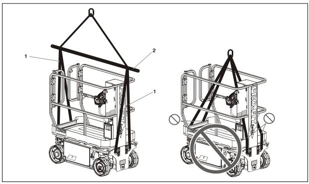
Figure 4-14. Lifting Using Spreader Bar.
