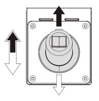
**Drive** - The drive and lift switch (*item 4 on the Platform Control/Indicator panel - Figure 3-8.*) must be selected prior to moving the control handle. After selecting the drive function, engage the trigger switch lever, then move the control handle forward to drive the machine forward or move the control handle backwards to drive the machine backward.
