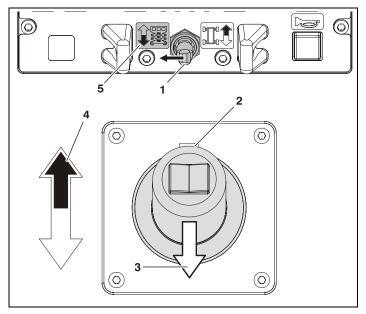
Figure 4-6. Raising Platform From Platform Control
