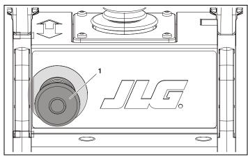
Figure 4-4. Platform Control - Emergency Stop Switch
