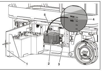
Figure 6-1. Hydraulic Oil Check Procedure
