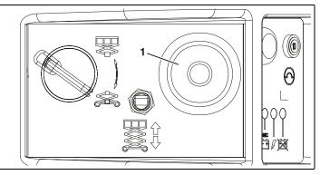
Figure 4-3. Ground Control - Emergency Stop Switch
