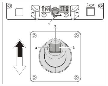
Figure 4-9. Steering from Platform Control
