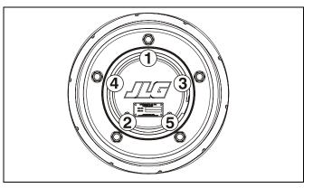
Figure 6-3. Wheel Lug Nut Tightening Sequence
