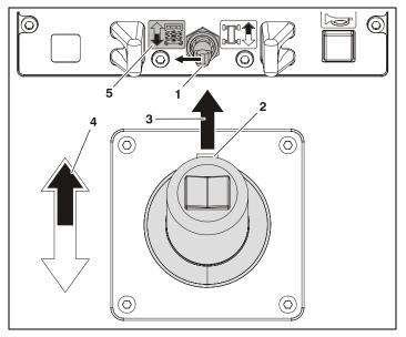
Figure 4-8. Lowering Platform From Platform Control
