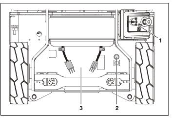
Figure 4-15. Electric Brake Release.
