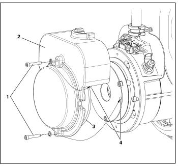
Figure 4-16. Brake - Manual Disengage.
