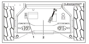
Figure 4-12. Location of AC Inverter ON/OFF - Toggle Switch
