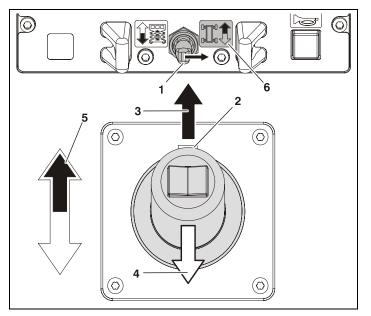
Figure 4-10. Driving Forward from Platform Control
